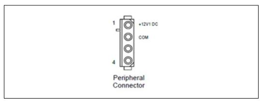
Table 4-7: Peripheral Connector Pin-out
