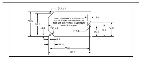
Figure 13-5: Recessed Fan Mounting
