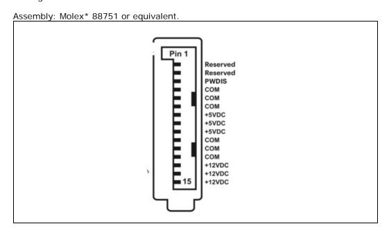
Table 4-10: Serial ATA\* Power Connector Pin-out
