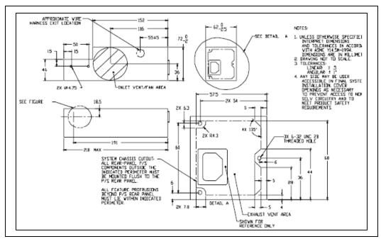
Figure 11-3: PSU Slot Feature Detail
