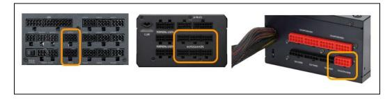
Based on the amount of current that is needed to support a specific current (power) level, the guideline to follow is 6-8 Amps per pin. This is based on 18 AWG wire and a solid connector pin. Based on this recommendation, the CPU power connectors can be applied:
