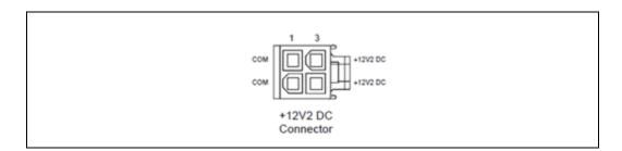
Table 4-3: +12 V Power 4 pin Connector Pin-out
